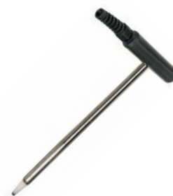
VPT SOIL for direct measures on soil cod: 50004082
